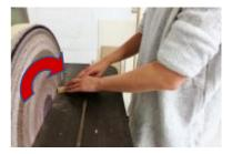
(When the disc rotates to the right, hold workpieces only on the right sight of the disc When the disc rotates to the left, hold workpieces only on the left sight of the disc) • Material that must NOT be ground
