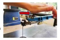
(Caution: If the clamping block does not slide straight into the holder at the top, the saw blade is too loose or too tightly clamped and can tear or cause poor cutting results)
