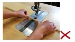
Only change the saw blade when the machine is completely switched off
