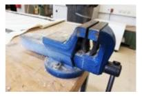
If the material is soft, a layer of wood should be used, as the surfaces of the vice can leave marks
